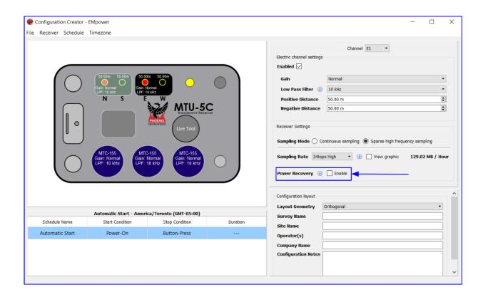
If many months later someone tries to use this MTU/RXU with a regular config file (even if it does not request power recovery), the receiver will try to turn on automatically after a good battery is connected, since the flag of power recovery is still active until the receiver boots with the new SD card.
